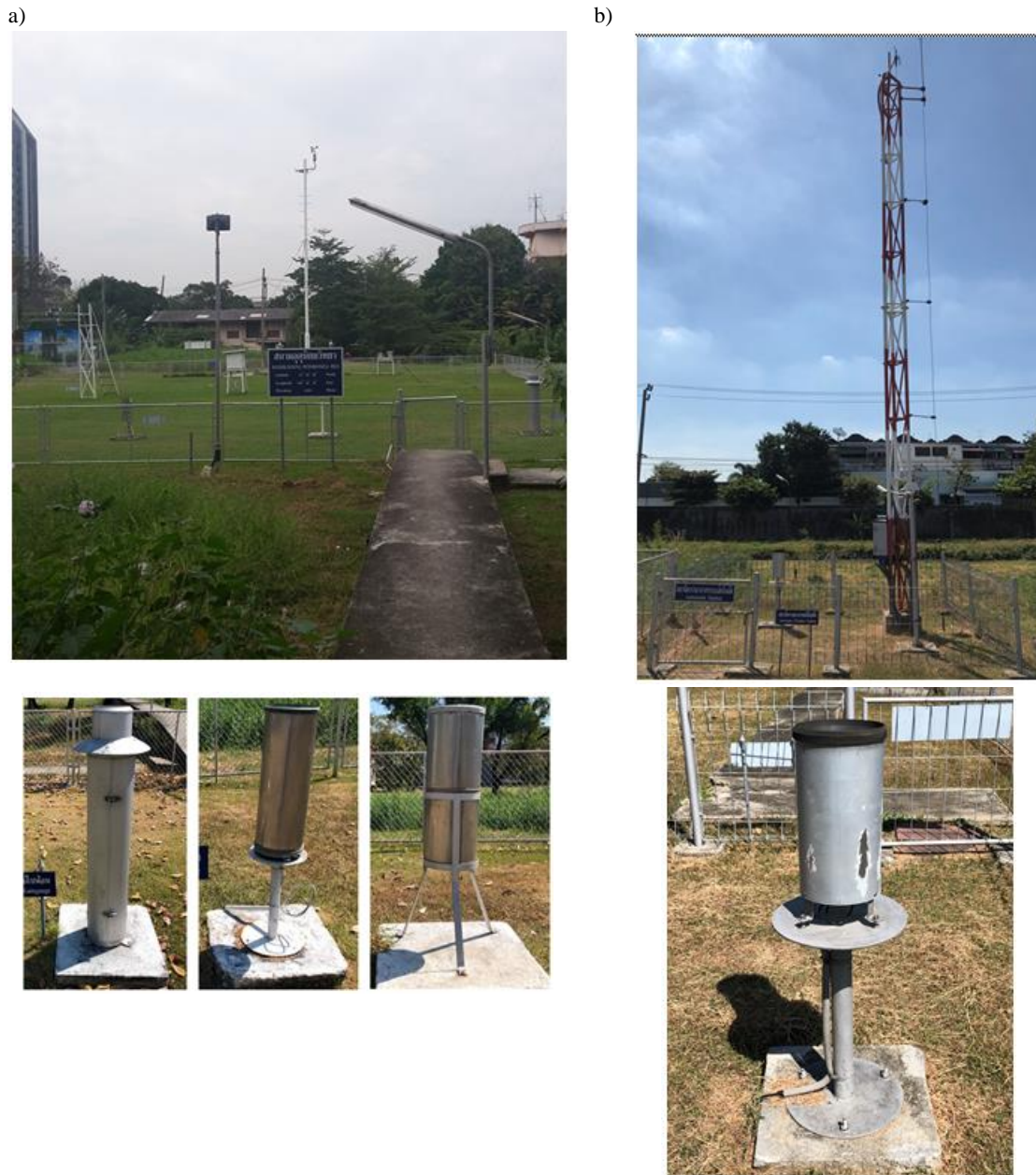
Figure S1. a) Standard gauge and b) auto gauge at the Bang–Na weather station of the TMD.
